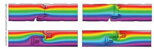
**ABOVE** An SR&eD tax credit partially funded an experiment conducted by Coolearth Architecture to improve the accuracy of energy models in their design process. using TheRM software, the firm modelled the flow of heat at the joints of two different insulated metal panel products to predict the effect of thermal bridging.
